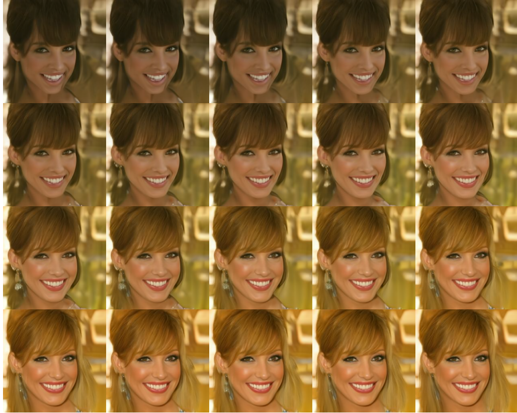
Figure 5.6: Sample transformation when optimizing the pretrained google/ddpm-celebahq-256 model using JPEG incompressibility as the reward function. The top-left image shows a sample generated by the pretrained model. Moving from left to right and top to bottom, the sample is regenerated from the same initial noise after each update of the model’s parameters. The final result of the finetuning process is shown in the bottom-right image.
