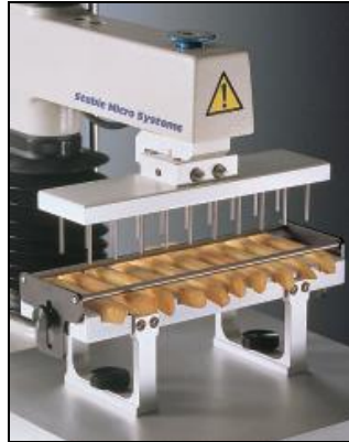
Figura 2.3: Texturómetro TA-XT2i (Stable Micro Systems, Surrey, UK)
