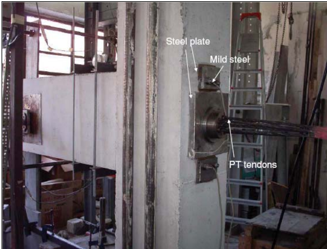
PCI Journal "Behavior of Unbonded Post-Tensioned Precast Concrete Connections with Different Percentages of Mild Steel Reinforcement" (ref. 15)
