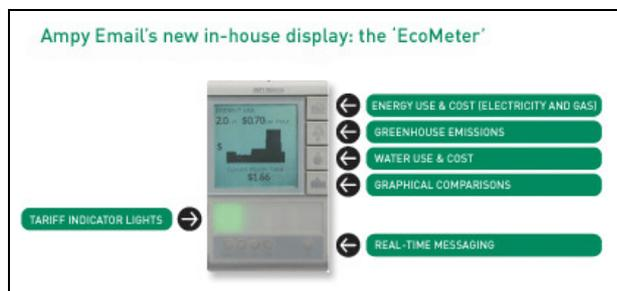
Figura 32: Visor “Ecometer” de Ampy (Landis+gyr Holding)
