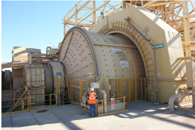
Figura 2.2-1 Molino SAG FLSmidth gearless, ring motor ABB
