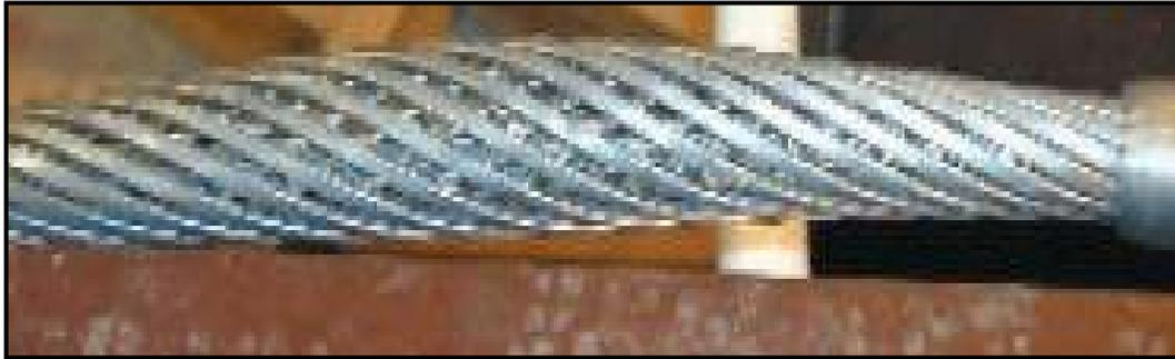
**d) Conductor tipo ACCR (Aluminum Conductor Composite Reinforced) 3M<sup>MR</sup>**
