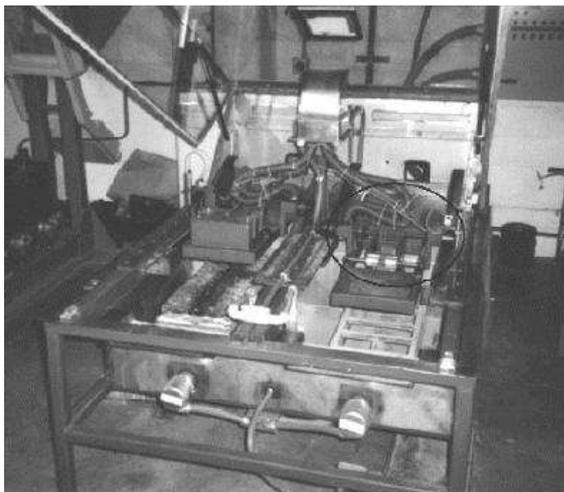
**Figura 9: Purdue University Laboratory Wheel- Tracking Device.**
