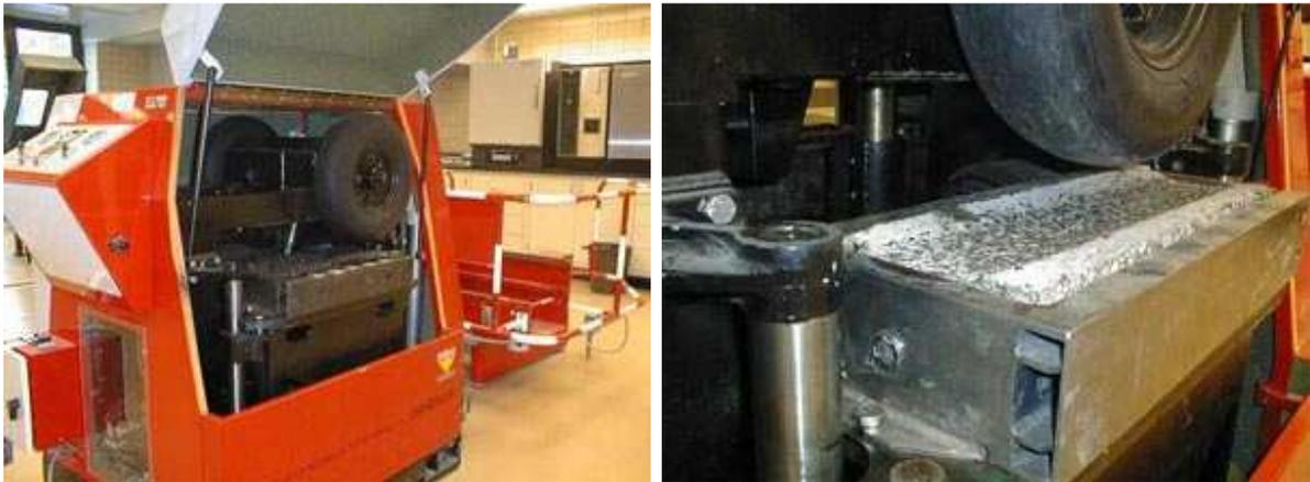
Figura 6: French Pavement Rutting Tester
