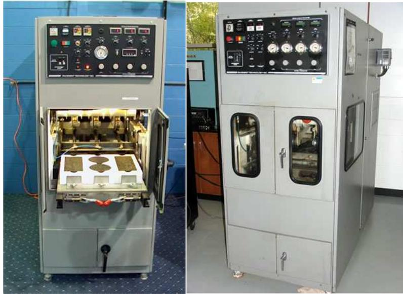
Figura 7: Asphalt Pavement Analyzer.
