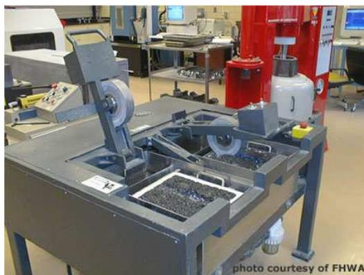
**Figura 8: Hamburg Wheel-Tracking Device.**
