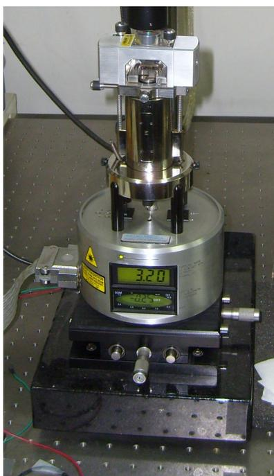
Figura 3.1: Microscopio Digital Instruments Nanoscope IIIa
