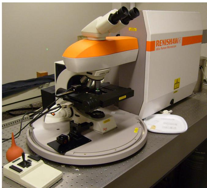
Figura 3.5: Microscopio Raman Renishaw inVia
