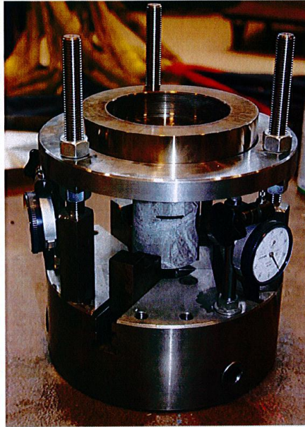
Figure 4. Photo of the “glue device” (with lower loading platen in upper part of picture).
