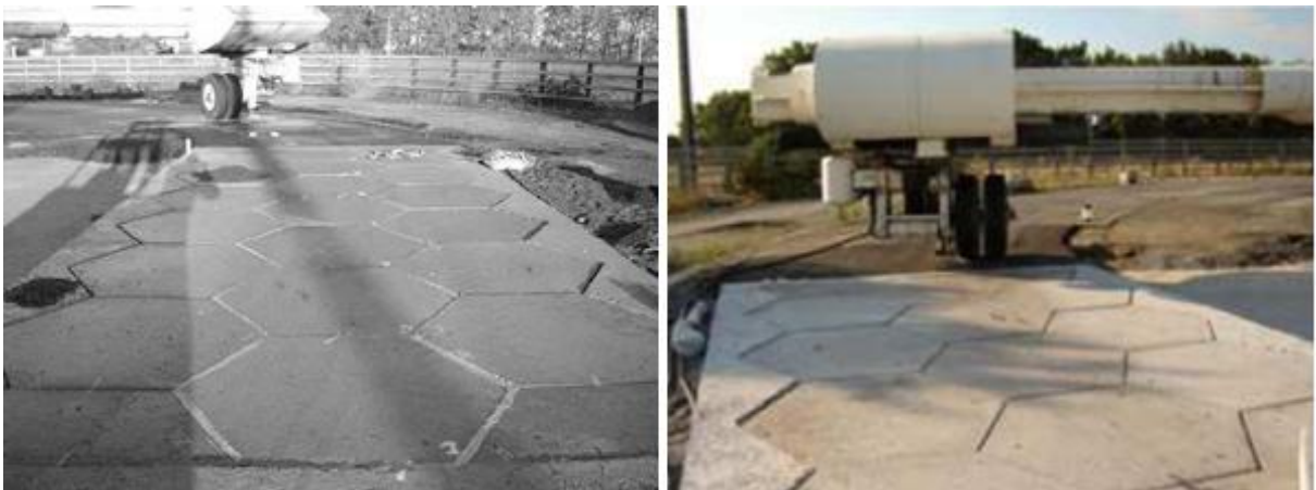
Figura II.39. Ensayo de cargas cíclicas mediante el LCPC Accelerated Load Testing Facility.
