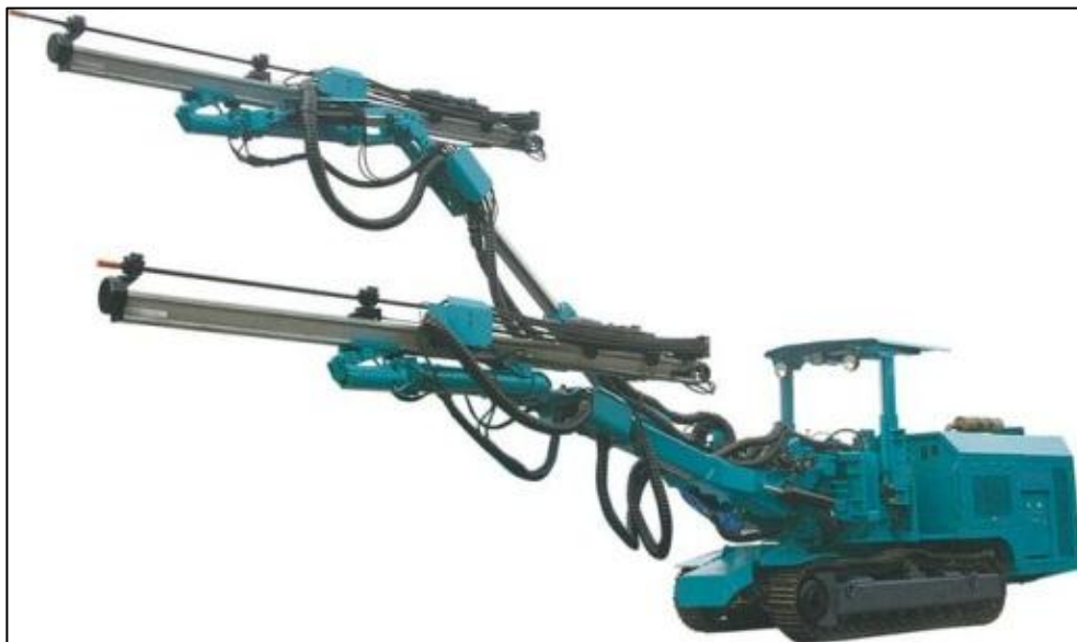
Figura A - 2. Perforadora Jumbo marca Sunward Model SWC452
