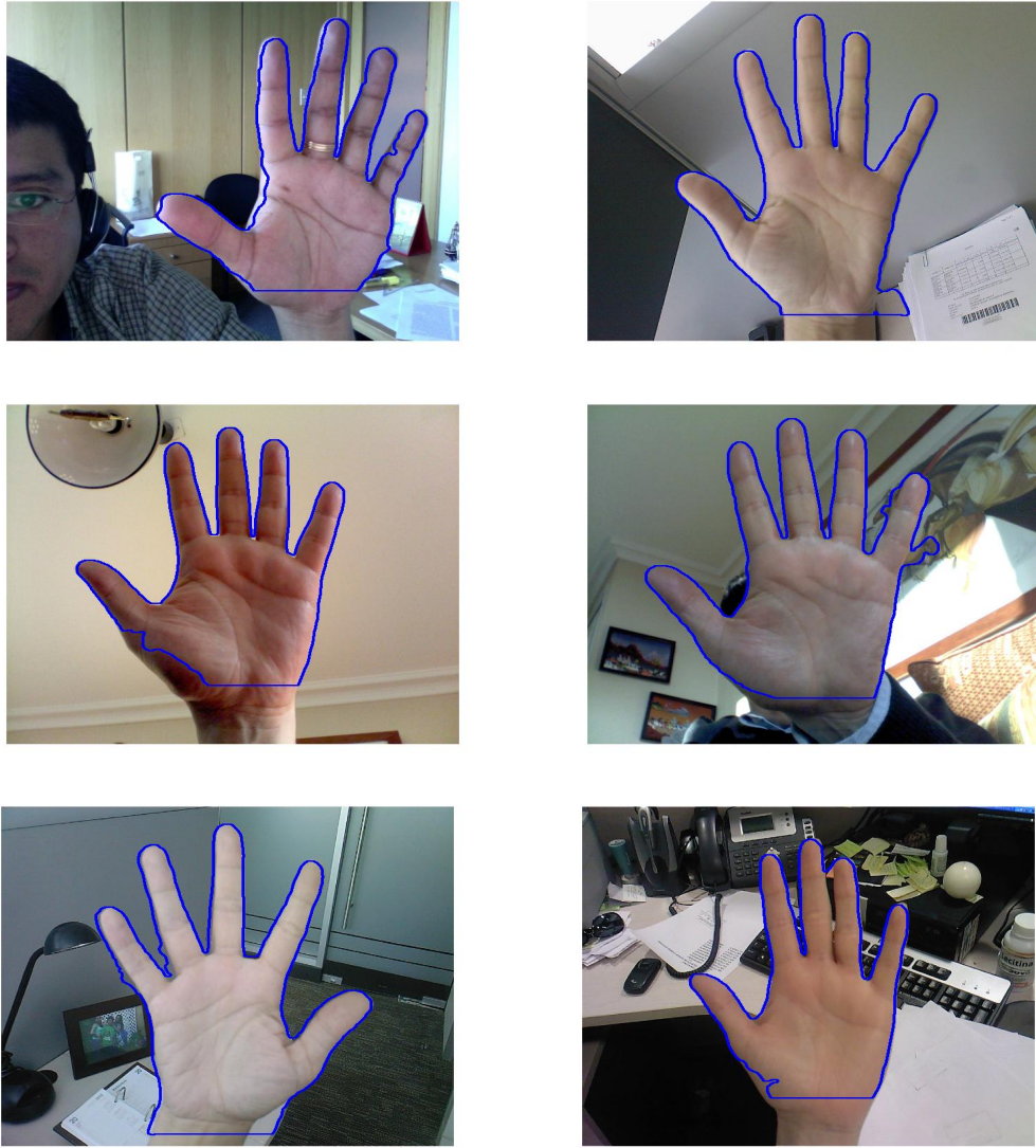
Figure 6.23: Examples of hand segmentation using our proposed approach.
