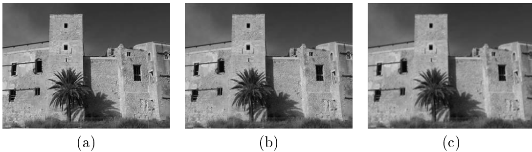
Figure 2.3: (a) Original image. (b) Image convolved using a 3 \times 3 kernel with \sigma = 0.5 . (c) Image convolved using a 3 \times 3 kernel with \sigma = 1 .
