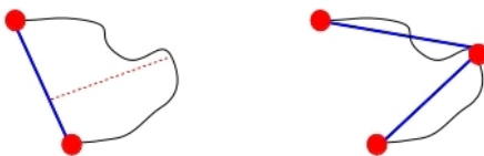
Figure 6.5: Approximating a stroke by a set of straight lines.
