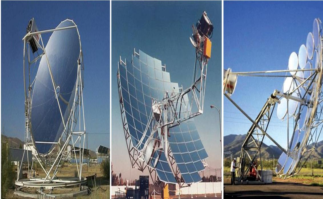
**Figura 15. “Concentradores Solares Stirling” [6][15]**
