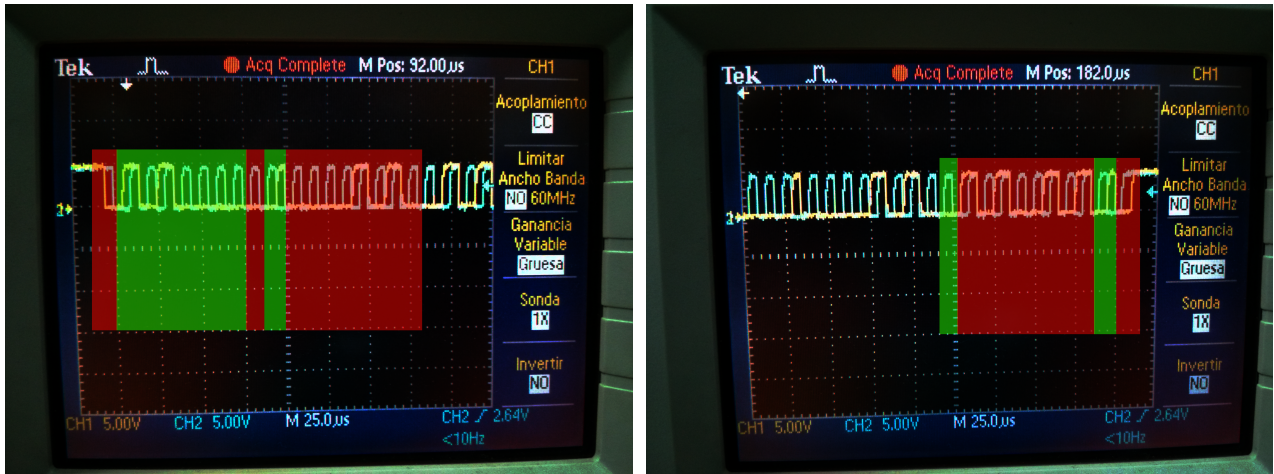
Figure 4.3: Data (yellow) and clock (blue) signals for writing into the memory. The different parts of the signal from left to right are: (i) Start condition, (ii) slave Address, (iii) write bit, (iv) slave acknowledge, (v) register address, (vi) slave acknowledge, (vii) register data (sent by master), (viii) slave acknowledge and (ix) stop condition.
