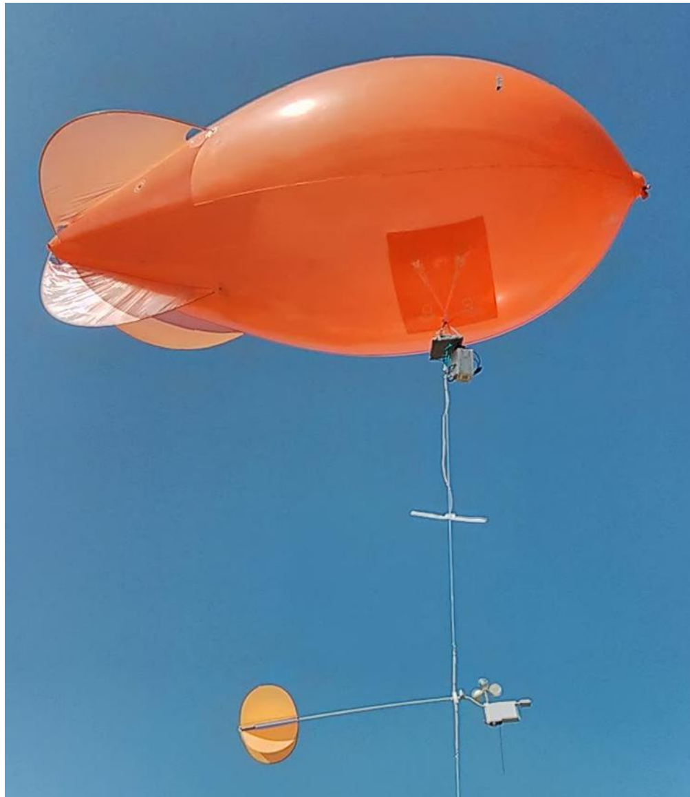
Figure 4.10: Setup of the captive balloon test. The elements in the photo from top to bottom are: balloon, aethalometer, radiosonde under test, radiosonde's antenna, Air radiosonde.
