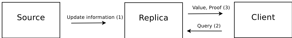
Figure 3.1: Three-party model: (1) The Source sends the updates of the database to the Replica with additional cryptographic values. The Replica convinces the Client that the answer to the query (2) is valid using a proof (3).
