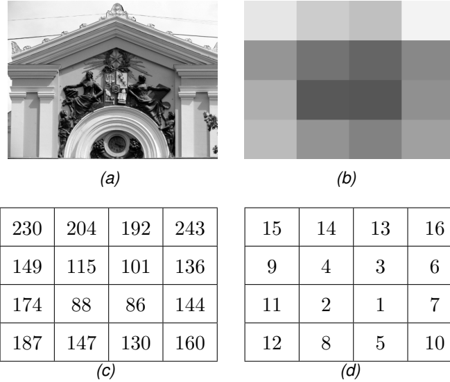
Figure 2.9 – Ordinal Measurement 4 \times 4 descriptor. (a) Sample gray image. (b-c) Average intensities for the image divided into 4 \times 4 zones. (d) Rank assigned to each zone.
