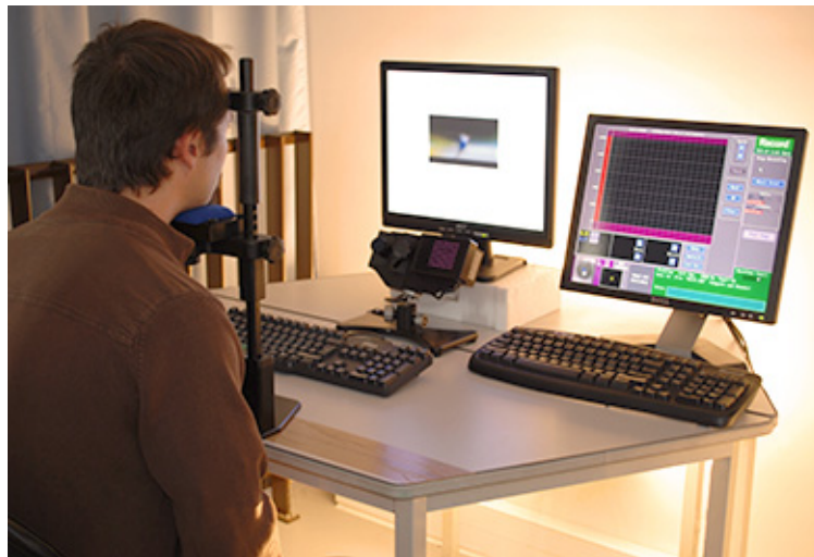
Figure 4.1: Eyelink 1000 layout with a subject
