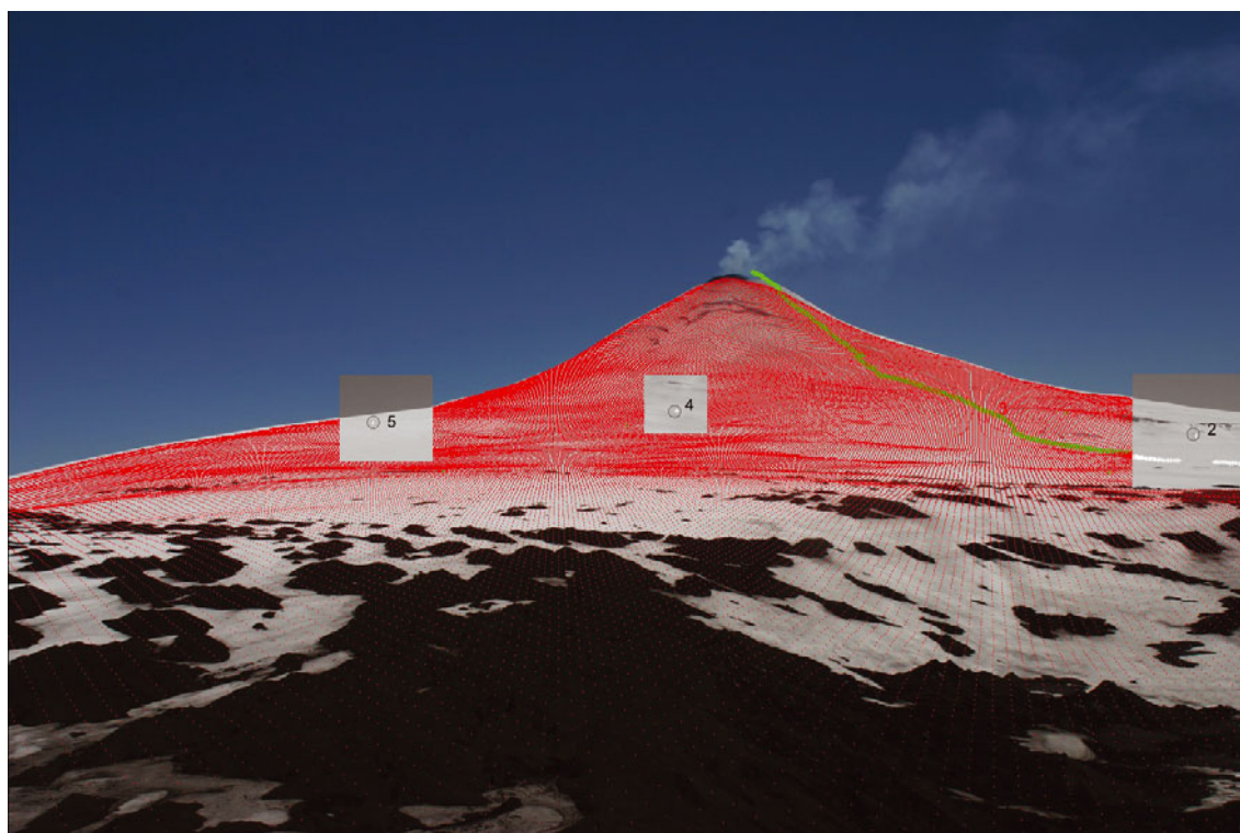
Fig. 4. Image of Volcán Villarrica and superimposed perspective projection of the DEM. Every red dot corresponds to a gridcell in the DEM. Circles in the insets show the location of precise ground-control points. In the terrain these were marked by flags visible in the original high-resolution photograph.
