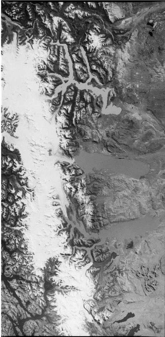
Fig. 5. An example of a declassified CORONA satellite photograph of the Southern Patagonian Icefield. The full resolution of the data is quoted as 6 ft ( \sim 2 m) and stereo pairs were obtained at 25 ft resolution from February 1962, at 9 ft resolution from August 1963 and 6 ft resolution from September 1967 until May 1972.
