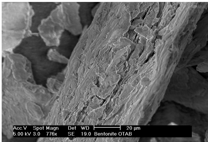
FIGURE 1 Scanning electron micrograph of [Bentonite(OTAB) 0.42 · 1.9(H 2 O)].
