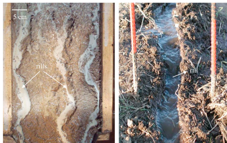
Figure 2. (left) A rill formed in the IIHR-Hydroscience and Engineering laboratory. (right) The formation of rills in a hill [after Mancilla, 2004].
