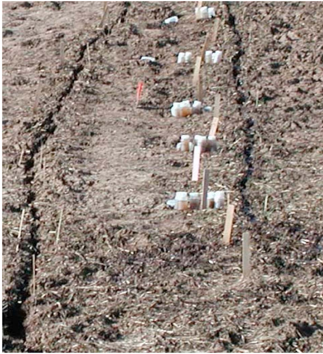
Figure 16. The Mancilla rills in the Palouse. Posts indicate sampling locations (see sampling bottles placed at the measurement locations) [after Mancilla, 2004].
