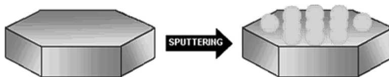
Figure 1. Representation of the deposit of the CuNPs on the plane (001) crystal of the IC.
