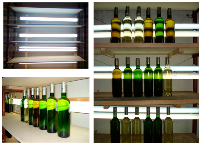
Figure 1. Photograph showing the open cabinets with the arrangement of the fluorescent tubes and bottles during the 8 months of storage.
