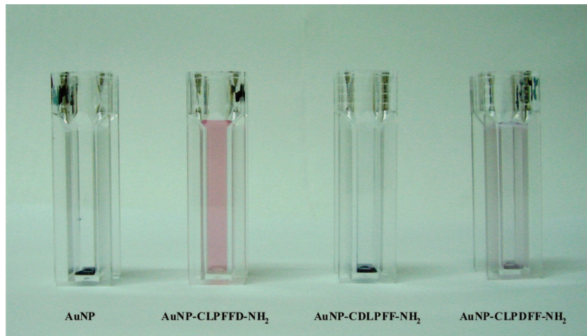
Figure 7. Photographs of colloidal solutions of bare AuNP and conjugated AuNP after incubation in ACSF for 48 h at 4 °C (AP, 0.05 \pm 0.01 for AuNP-CLPFFD-NH 2 ; for bare AuNP and other conjugates, the AP could not be determined because the sample was totally precipitated).
