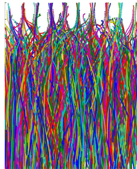
Fig. 8 Recovered particles trajectories after the analysis of 199 frames. The color is used to better visualize individual particle trajectories
