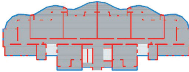
Figure 4. Typical floor plan (red = walls, blue = beams).
