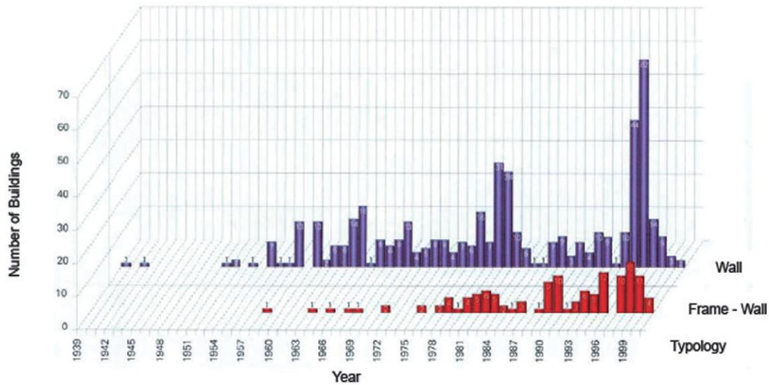
Figure 6. Variation of the construction system in Chile with time (Instituto del Cemento y del Hormigón de Chile, 2002).
