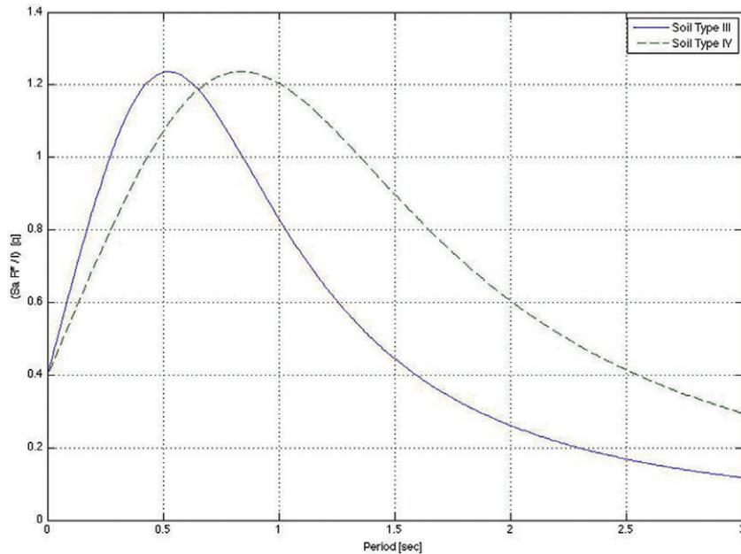
Figure 3. Nch433.Of96—elastic design spectrum for the Concepción area.
