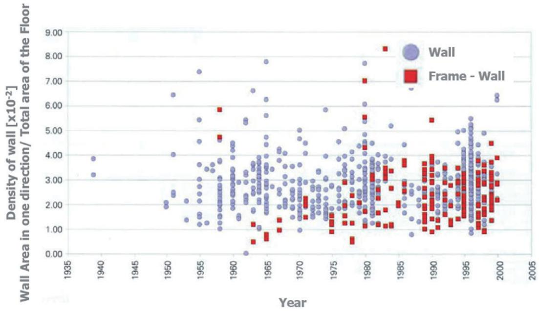
Figure 8. Density of walls at one floor as a function of time (Instituto del Cemento y del Hormigón de Chile, 2002).
