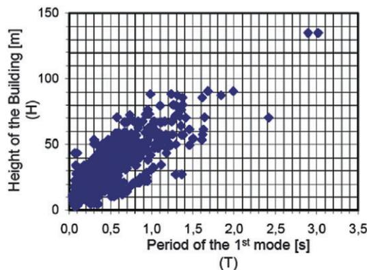
Figure 7. Relation of height of the building versus fundamental period (Guendelman *et al.*, 2000).
