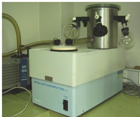
**Figura N° 16:** liofilizador Savant Refrigerated Condensation Trap R 100.
