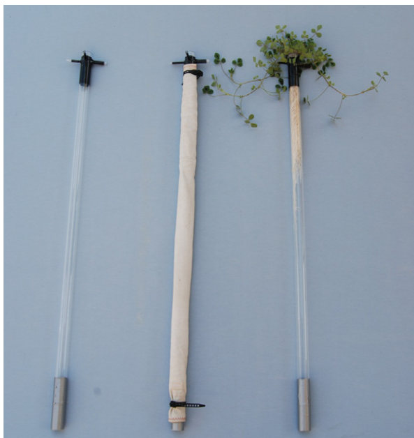
Figure 8. Glass tubes functioning as a root/nodule compartment that can be sealed airtight and individually aerated and supplied with a circling nutrient solution flow.
