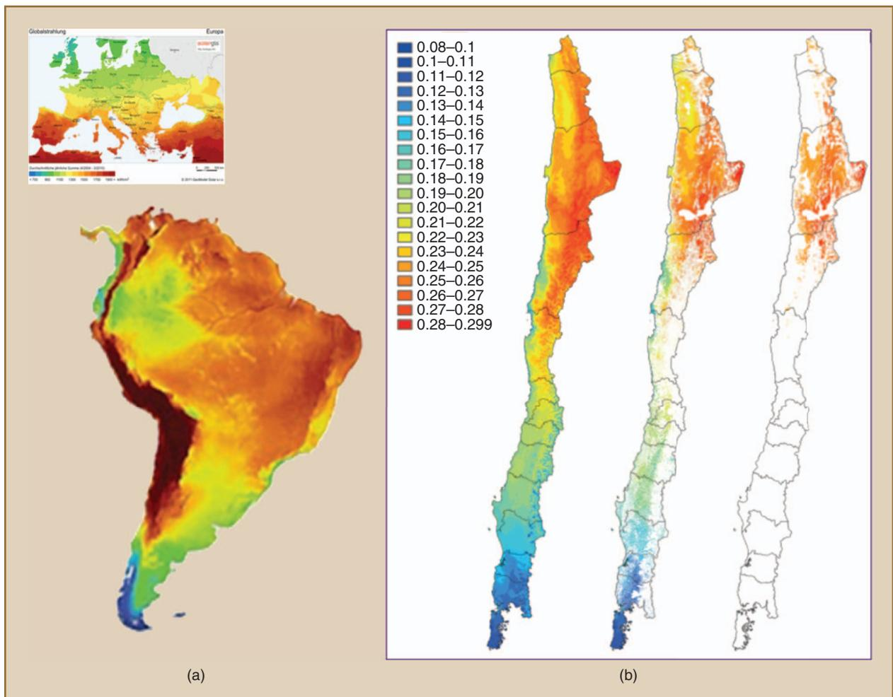
**figure 1.** Chile's solar energy potential: (a) compared with that of Europe and (b) annual plant factor distribution, with various constraints added moving from left to right (source: Chilean Energy Ministry).
