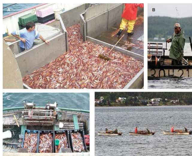
Figure 5. Gear types used in the Illex illecebrosus fisheries. (A) The squid catch of a USA bottom trawler (a freezer vessel) is pushed from the “pen” area, shown here, to a conveyor belt for sorting on deck prior to packing and freezing the catch in the hold. (B) A fisherman manually operates a jig reel while fishing for squid near the Newfoundland coast. (C) A view from the dock of jig reels used in the small-boat (4–14 m in length) squid fishery off Newfoundland and a day's catch. (D) Fishermen jigging for squid in a Newfoundland embayment. Photograph credits: (A) Lisa C. Hendrickson; (B) downhomelife.com.
