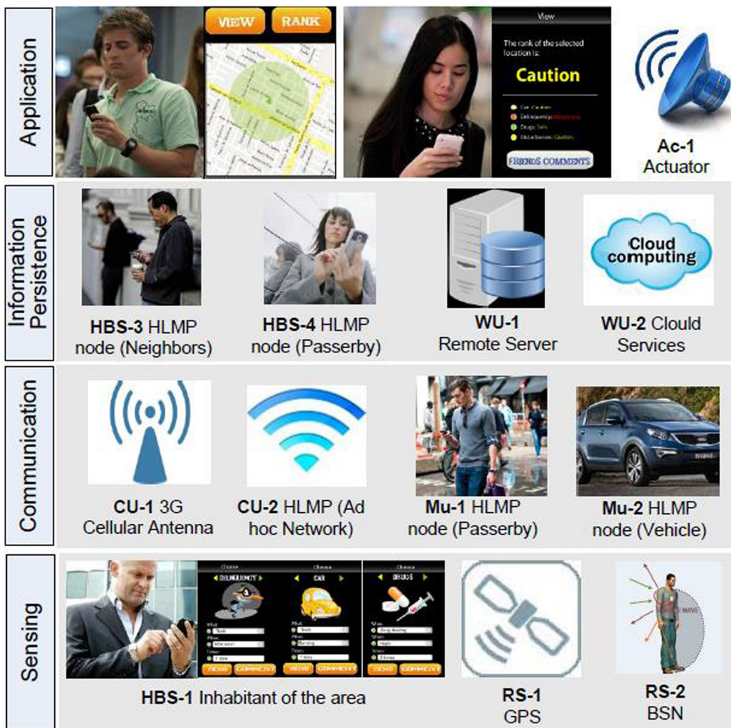
Figure 1. Layered architecture of the HWSN that supports the PG system.
