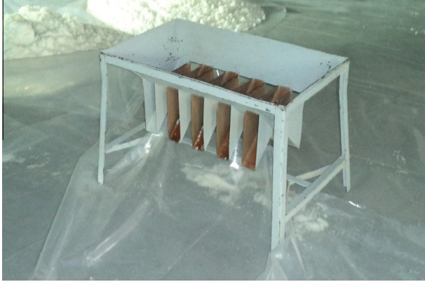
Fig. 4. Sample splitter used to quarter the bischofite.
