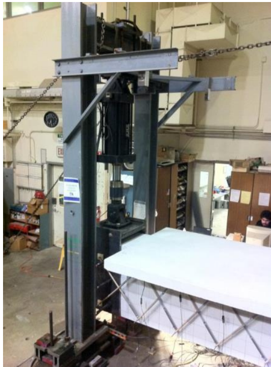
Figure 3.12: Loading Frame with Actuator (Lemnitzer et al., 2013).
