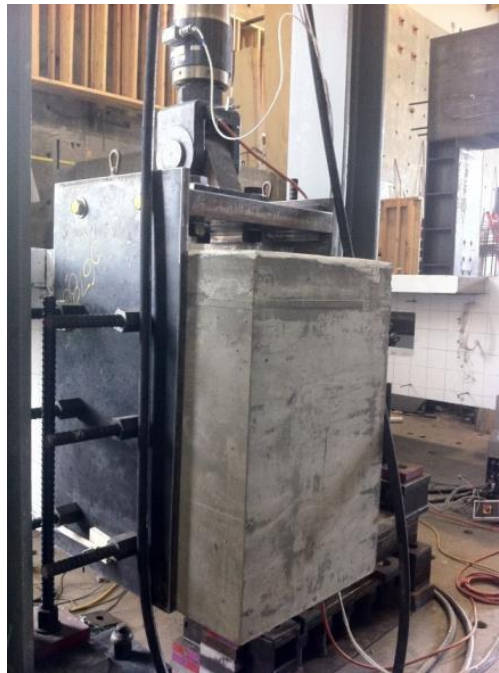
Figure 3.13: Plate system anchored to the specimen (Lemnitzer et al., 2013).
