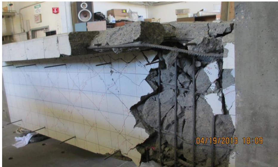
Figure 3.21: Specimen 7 after test completion, plastic hinge accompanied with rebar buckling, (Lemnitzer et al., 2013).
