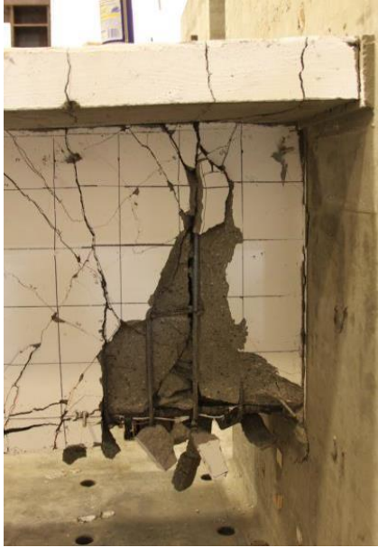
Figure 3.18: Plastic hinge at beam/block interface (Specimen 6), (Lemnitzer et al., 2013).
