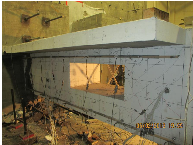
Figure 3.17: Specimen 2 at test completion with plastic hinge at the left of the picture and the undamaged opening at the center, (Lemnitzer et al., 2013).
