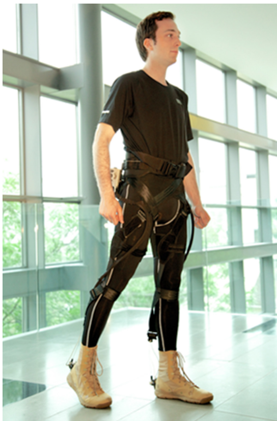
[3] Soft Robotic Exosuit, 2014, Exoesqueleto robótico. ©Harvard Wyss Institute, Harvard Biodesign Lab.
