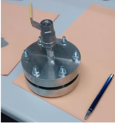
Figure 9: a batch reactor vessel used in the experiments
