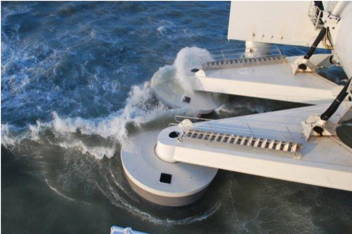
Figura 2-14: Wave Star escala 1:2 [16]
