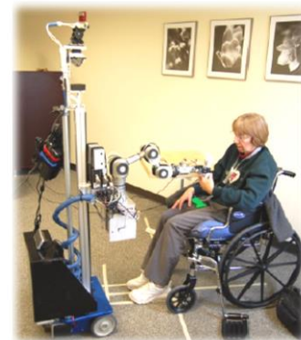
Ilustración 10: Robot El-E asistiendo a paciente con ALS. “Hand It Over Or Set It Down: A User Study of Object Delivery with an Assistive Mobile Manipulator”, Sang Choi et-al (2009).
