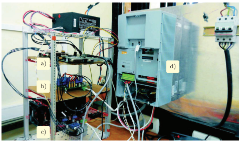
Fig. 6. Laboratory setup. (a) DSP+FPGA+FO interface. (b) Current sensor. (c) 2L-VSI. (d) Induction machine converter.
