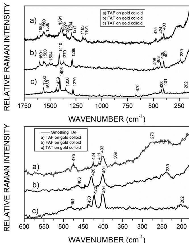
Fig. 3. SERS spectra of a) TAF, b) FAF and c) TAT, on gold nanoparticles, in the 1800–200  $\text{cm}^{-1}$  region (top) and 600–200  $\text{cm}^{-1}$  region (bottom).
