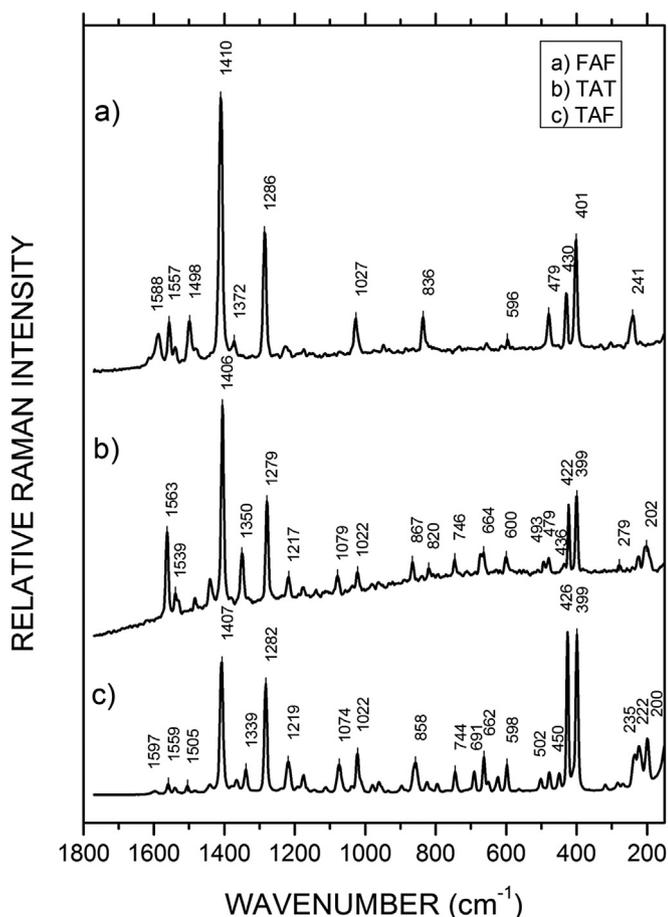
Fig. 2. Raman spectra of the solids of the cruciform systems: a) FAF, b) TAT and c) TAF.
