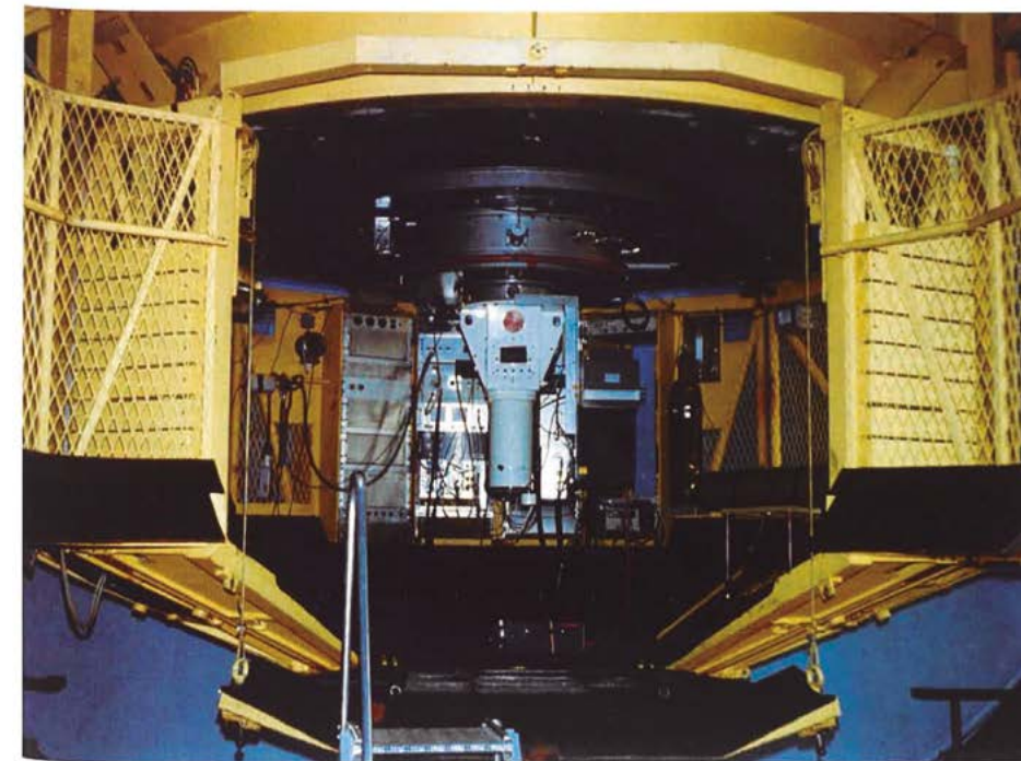
The Cassegrain cage of the 3.6 m telescope with the Boller and Chivens spectrograph. (Photograph by J.P. Swings.)
