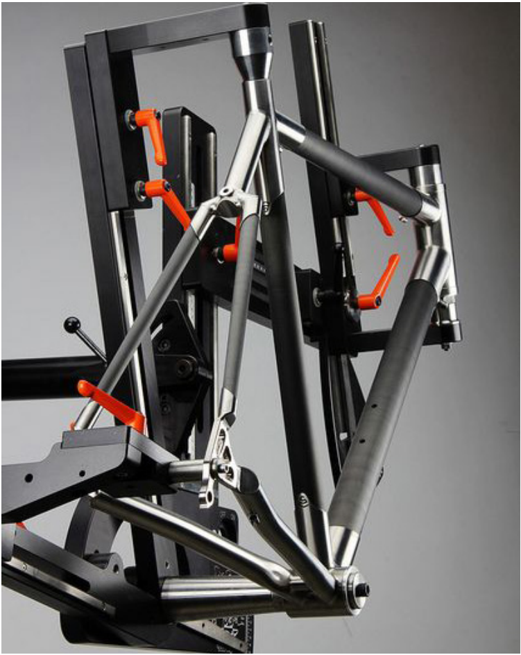
Imagen 1. Matriz de armado Firefly Bicycles. Fuente: http://www.flickr.com/photos/fireflybicycles/with/8540312278/ , firefly bicycles (bicycles, 2001)
