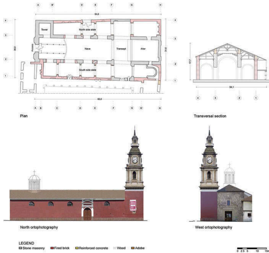
Figure 1. Plans, section and elevations of San Francisco in its current state, with information of the main building materials.
