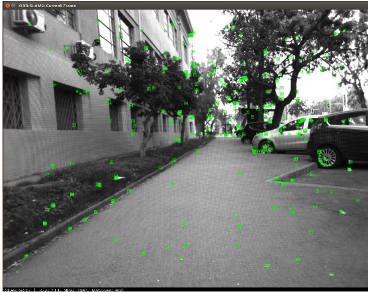
Figure 4.11: Image used in ORB-SLAM. The green squares represent the points detected with the ORB algorithm.
