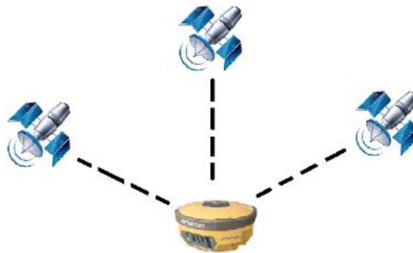
Figure 2.2: Triangulation GPS process.
