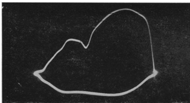
Fig. 5. 0.04 ml 10^{-2} M U(VI) in 6 ml TEA (0.1 M)—citric acid (0.1 M) in 3 : 3 proportion (pH = 4); d.c. = 3 mA; a.c. = 0.15 mA.
