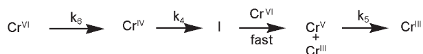
Scheme 2 \text{Cr}^{\text{VI}} \rightarrow \text{Cr}^{\text{III}} reduction pathway used to fit the experimental absorbance data; I = very reactive intermediate.
