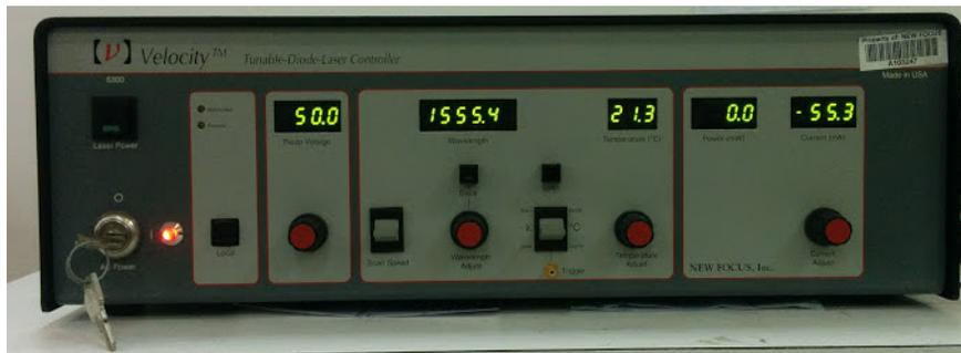
Figure A.2: Velocity 6300 control panel.
