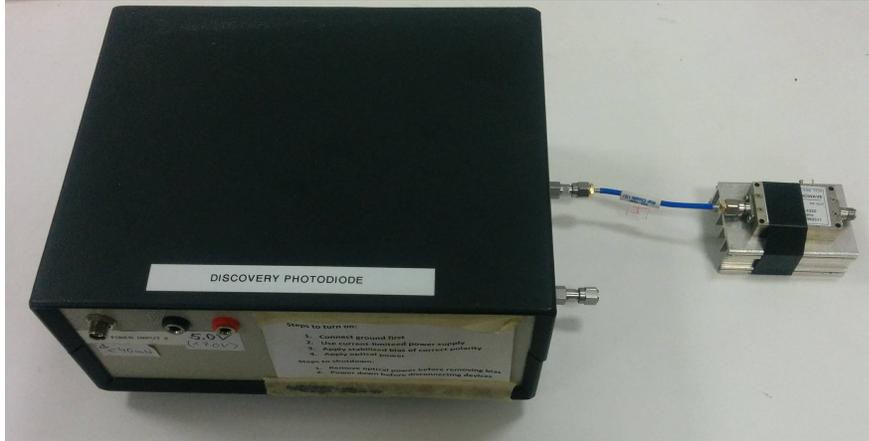
Figure A.6: Photodiode and low-noise amplifier (LNA) [38].
