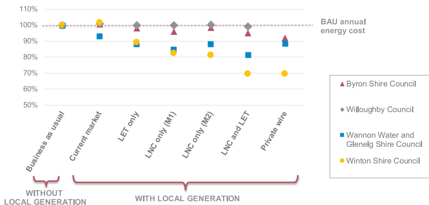
Fig. 1. First year impact on proponents (total energy costs). Note 1: LNC only (M1) uses the volumetric method of calculation for the LNC, while LNC (M2) uses the combined volumetric and capacity payment. The LNC and LET scenario includes the effects of LET and the LNC. In the table the average value of the LNC calculated using method 1 and method 2 has been used for the LNC and LET scenario, as the difference between the two scenarios is simply difference between LNC only (M1) and LNC only (M2).
