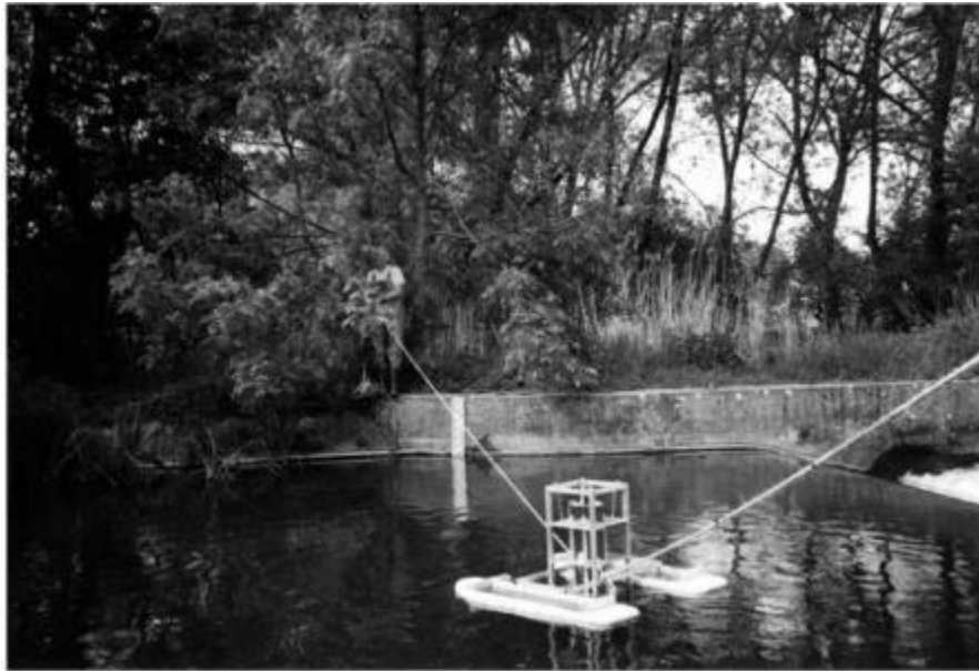
Figura 2.23: aforo mediante sensor ADCP (Acoustic Doppler Current Profiler).
