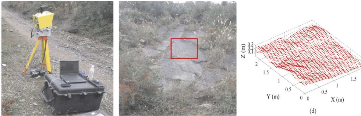
Figure A.7. LIDAR surface topography measurement process (Modified from Ge, 2015)
